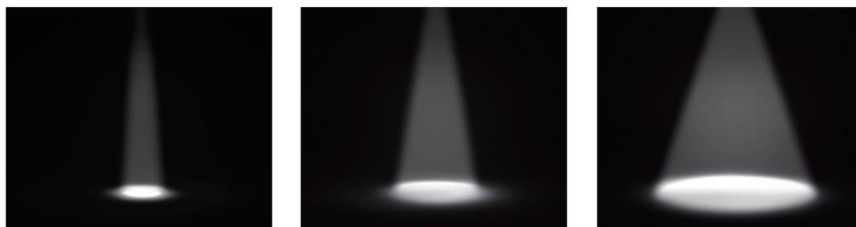
Light distribution angle can be adjusted from narrow (10°) to wide (30°) in SALIOT, which can set a selection area freely based on the irradiation symmetry and location, thereby optimizing lighting options for any application.
