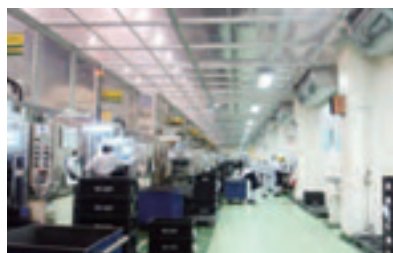
Working areas and passageways in the Rojana Plant are more effectively cooled by partitioning them off from the rest of the plant with panels
