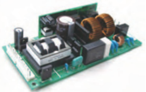
The new AC-DC converter that does not require heat sinks
