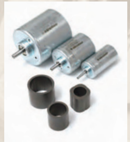
The advanced bond magnets developed by the team (foreground) and motors planned for future development (rear).
