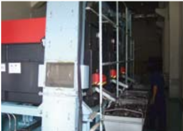
Equipment for recovery and compression of swarf
