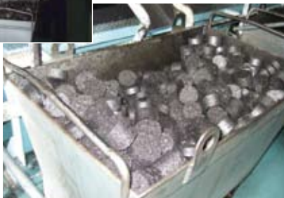
Equipment for recovery and compression of swarf
