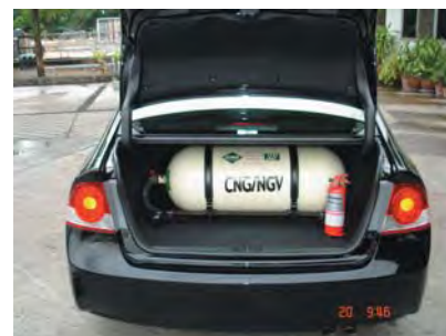
Gas tank installed on NGV
