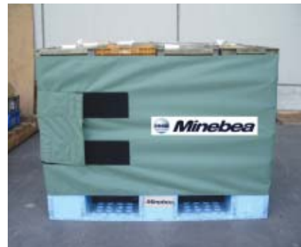
Result of improvement: Recyclable, reusable polyester strapping bands used to prevent load collapse. The bands can be reused approximately 1,000 times and at the end of their useful life they are recycled into fiberboard.
