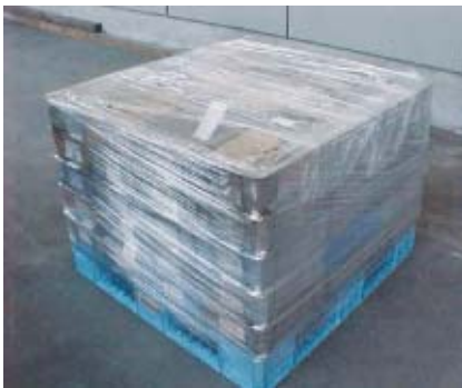
Polyethylene stretch film used to prevent load collapse
