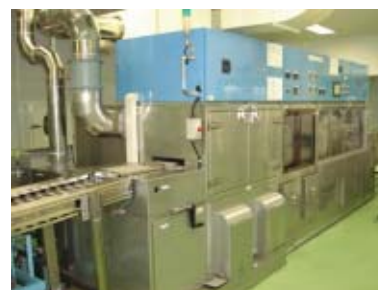
Cleaning facility that uses purified water, newly installed Shanghai Plant (China)
