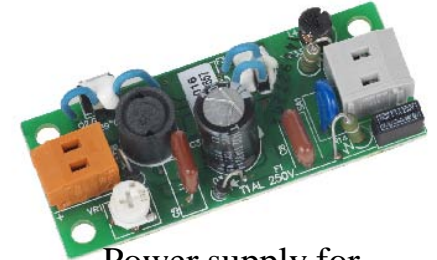
Power supply for LED lighting apparatus
