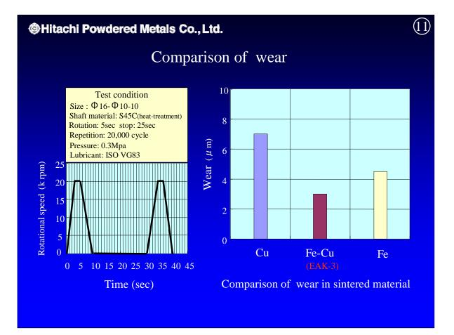
As one example, this data shows Nikkaloy EAK-3's friction resistance under repeated ON/OFF operations.
