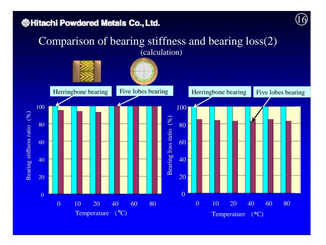
This figure compares bearing stiffness and bearing loss from the previous slide, expressing the relationship as a percentage. Bearing stiffness does not show any substantial change at different temperatures, but for bearing loss the figures for five-lobe bearings are close to 20% lower at all temperatures.
