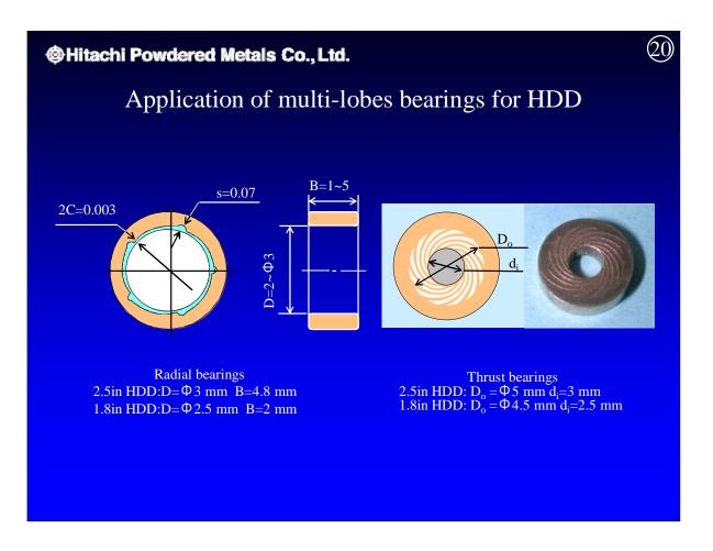
The bearing is designed with a minimum clearance of 3 microns, separation groove of 70 microns and bearing width of 1-5 mm.
