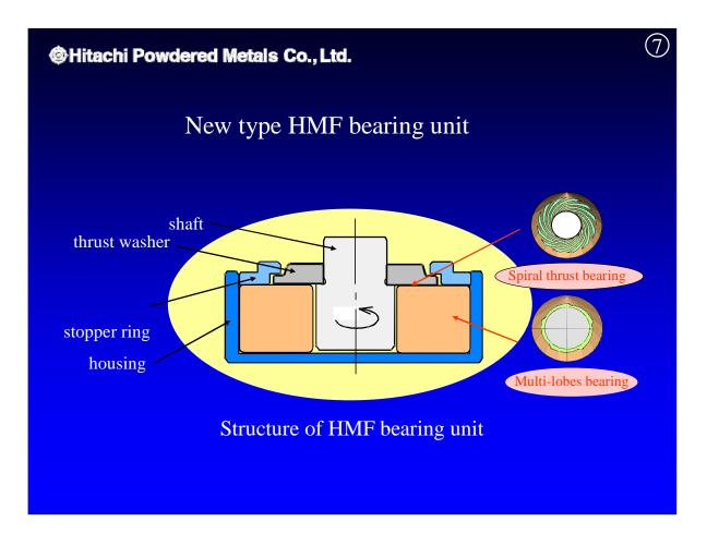
We collaborated with Minebea on the development of HMF type FDB units. The name comes from the initials of the two companies. We provide the bearing portion; Minebea assembles the bearing unit. The inside of the bearing portion is formed with multiple lobes. The thrust face has spiral dynamic pressure grooves for the bearing.
