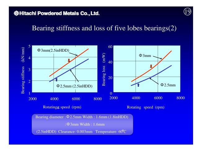
This figure provides a comparison under different RPM conditions. The red line shows the 3-mm shaft diameter used in 2.5-inch HDD spindle motors; the blue line, a 2.5-mm shaft for 1.8-inch HDDs. Optimum bearing stiffness and bearing loss values enable five-lobe bearings to be fully suitable for HDD spindle motors.
