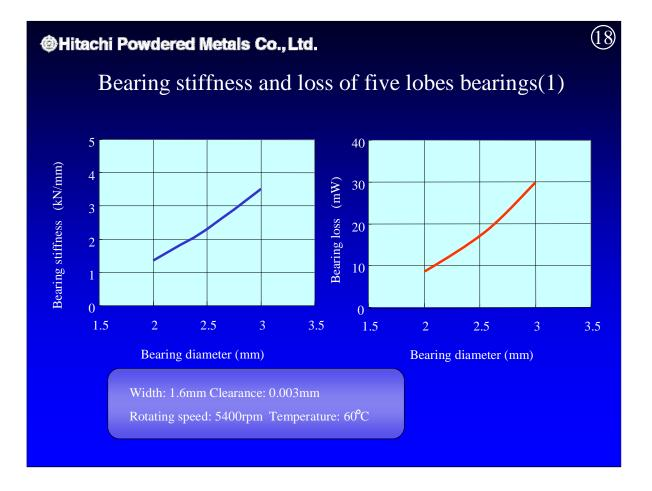
Bearing stiffness and bearing loss change according to the diameter of the bearing (shaft diameter). The smaller the shaft diameter, the lower the bearing stiffness, but the lower the bearing loss as well.
