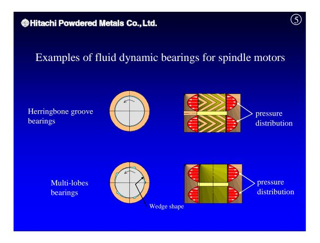
The most common FDBs used in HDD spindle motors today are what is known as the "herring bone type." As the name suggests, these bearings have grooves along the inside diameter of the bearing that are shaped like herring bones. By contrast, multi-lobe FDB have an array of evenly-spaced arcs ("lobes") running vertically along the inner diameter, with the wedging of the oil in the bearing openings generating dynamic pressure that produces stable revolution.
