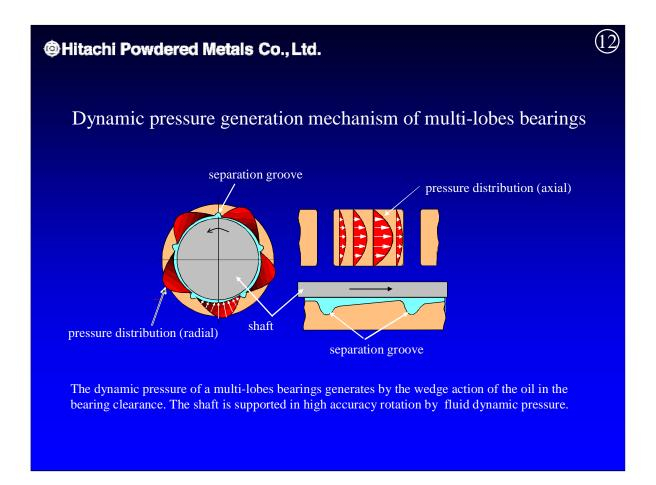
In multi-lobe bearings, when the shaft rotates counter-clockwise the wedge openings gradually narrow to generate the dynamic pressure. Then they open at the separation groove, and the next dynamic pressure is generated.
