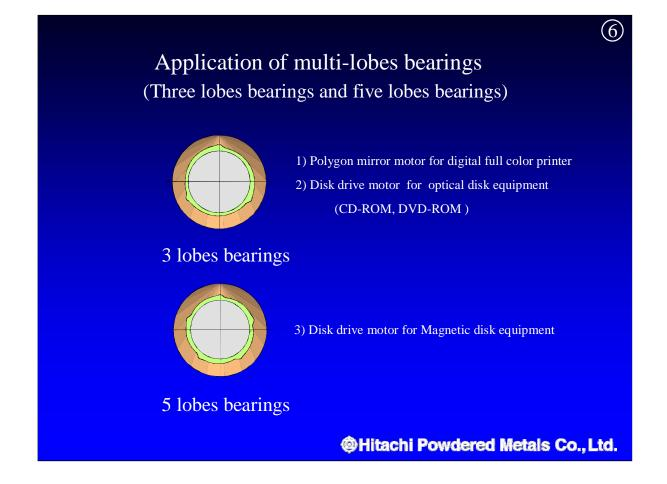
Three-lobe bearings are suited to high-speed, high-precision revolutions and are used in laser scanner motors and optical disc drive motors, among other applications. For the ultra-precise revolutions required by HDD spindle motors, we have developed five-lobe bearings (HMF). I will now explain about this bearing technology.
