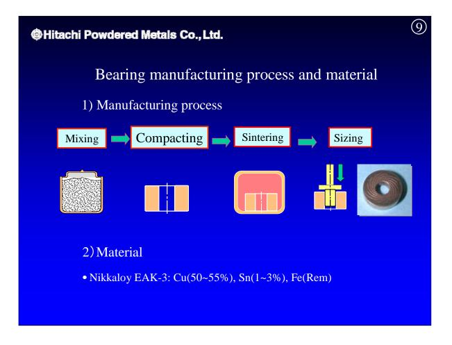
The manufacturing process begins by mixing the powder. We then use a metal mold to press-form the powder. This is followed by sintering to encourage metal bonding. Finally, the sizing process simultaneously forms the multiple lobes on the inside of the bearing and the spiral dynamic pressure on the tip. The result is extremely high-productivity and low-cost production.
