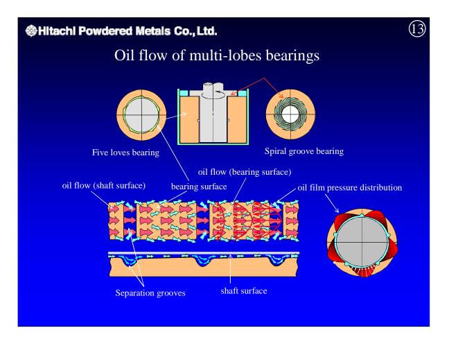
This development drawing of the inside of the bearing illustrates the oil flow. The blue arrows indicate the oil flow on the bearing surface; the red arrows also indicate the oil flow on the shaft surface. The shaft surface oil flows in evenly. The cross-section below shows how the oil temporarily builds up in the separation groove before flowing again.
