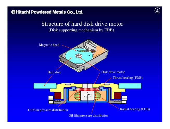
We recently announced a new HMF type fluid dynamic bearing (FDB) unit structured so that the dynamic pressure is generated on the inner surface and the upper thrust surface of the bearing. On the radial side, oil film pressure supports the shaft. On the thrust surface, oil film pressure in the upwards direction lifts up the entire thrust surface and causes it to slide.
