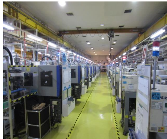
Molding line for connectors
