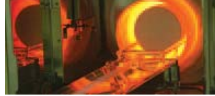
Placement of S0S structure in diffusion furnace
