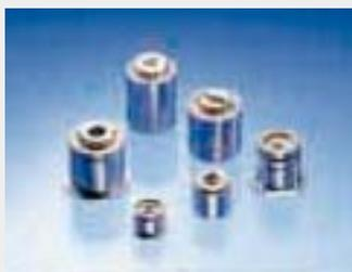
Pivot assemblies are fitted into the base of actuators to position HDD magnetic heads. Minebea enjoys the top share of the global market for these components. Standard pivot assemblies combine one or two ball bearings between a shaft and a graded sleeve.
