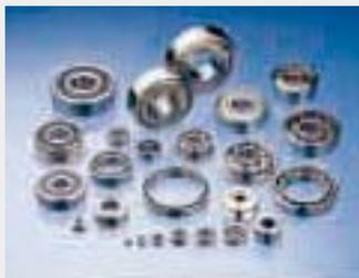
Each ball bearing comprises an outer ring, inner ring, balls, retainers, shields and snap rings. Essential to high-precision motors and other rotary components, ball bearings determine rotational accuracy. The average motor contains two ball bearings. Minebea manufactures more than 8,500 different types of miniature and small-sized ball bearings, most of which have external diameters of 22mm or less.
