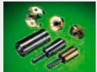
An integrated-shaft ball bearing has two raceways on the shaft, allowing the integration of the inner ring and shaft of two ball bearings. This facilitates more precise rotation than is possible with two independent ball bearings, making integrated-shaft ball bearings particularly suited to applications such as cylinder units for video cameras.
