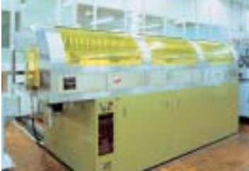
Water-based washing system
