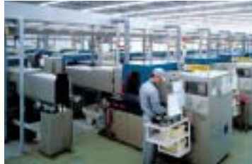
The Shanghai plant's cutting line is equipped with oil separators, which separate oil from metal chips, and oil collection ducts.
