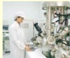
X-ray photoelectron spectrometers are used to investigate the surface chemistry and interactions of solid surfaces of metal and organic materials. The Thai R&D Center's X-ray photoelectron spectrometer enables researchers to determine, for example, whether metal discoloration is the result of oxidation or corrosion caused by chlorine, sulfur or other substances.
