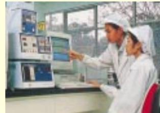
GC-MS is widely used to determine the chemical properties of substances. At the Thai R&D Center, researchers use the GC-MS to analyze gases released by the adhesives used in spindle motors, enabling them to identify gases that could potentially lead to functional problems for HDDs in field use.
