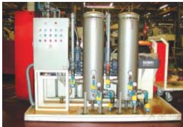
Dynamic filtration system (Fujisawa Manufacturing Unit)
