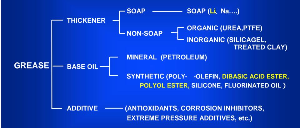
GREASE CONSISTS OF APPROX. 80% TO 90% OIL, APPROX. 10% TO 20% THICKENER AND APPROX. 1% TO 5% STIFFENER ADDITIVES.
