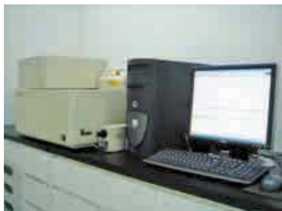
New X-ray fluorescence (XRF) spectroscope, used to detect the presence of hazardous substances in parts and raw materials purchased from outside suppliers (Bang Pa-in Plant)
